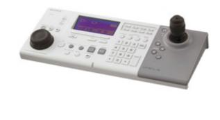
An optional RM-NS1000 System Controller - which connects to the NSR-1000 Series or a client PC via USB cable - allows the user to control multiple servers and cameras. A wide range of operations can be performed from this unit, including camera selection, Pan/ Tilt/Zoom (PTZ) with preset controls, snapshot capturing, video exporting, and event search and playback.
